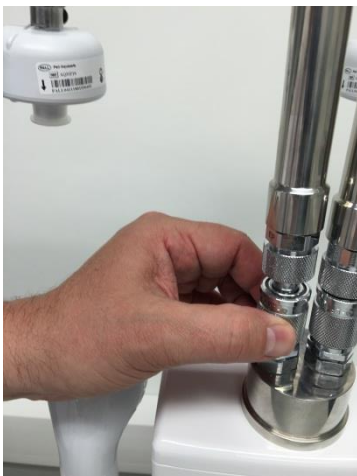
4. removable intake sheets - Press the shutter plug blades down -
