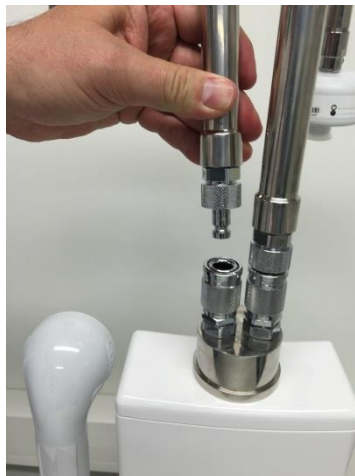
5. decoupling - Pull inlet arc -
